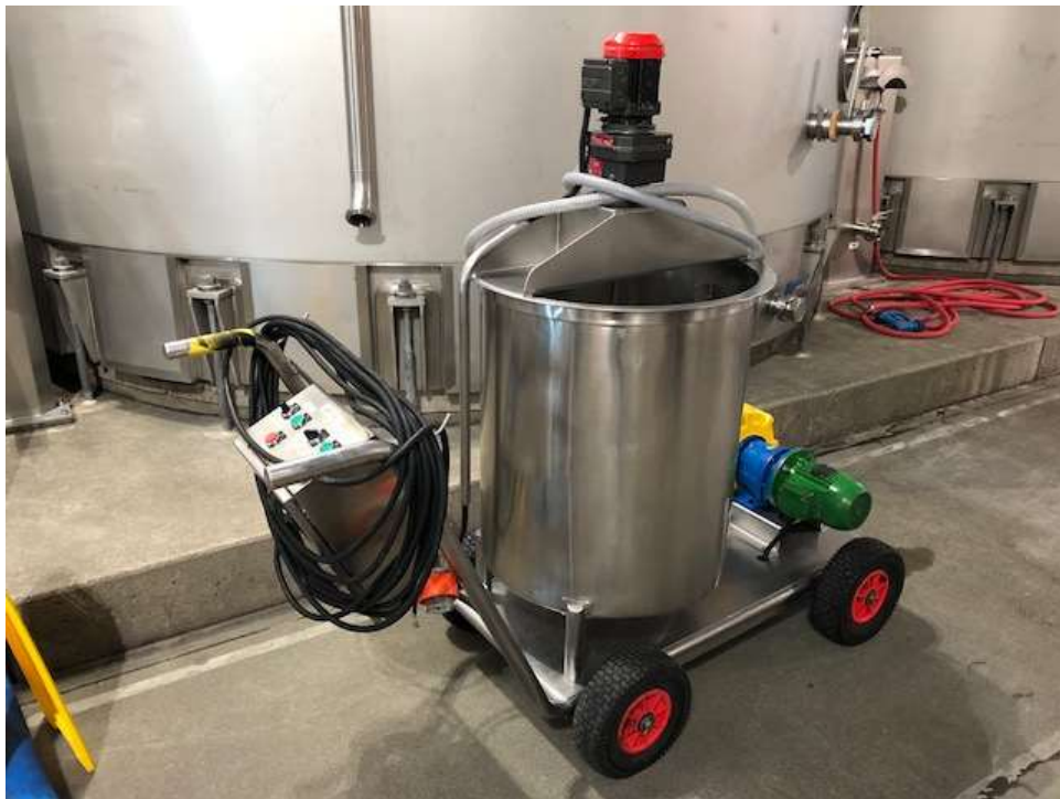
Mobile tank and mixer for making up additives in winery, complete with transfer pump.
